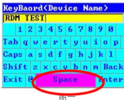
Please see above picture, this soft keyboard can be used by both touch screen and physical buttons. Using touch screen, just press the button to input;
