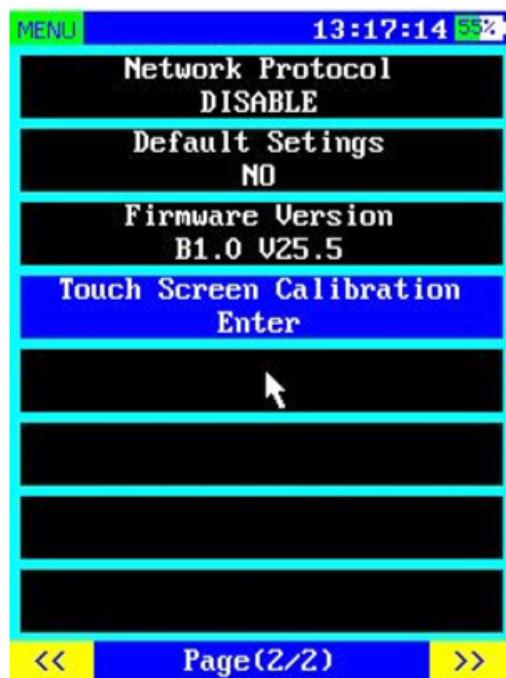
**Note:** The network function is only available in dmx output. If choosing to use network function, in *Send DMX* and *SEQUENCE* function options menu, the device will use the network to send dmx data at the same time(artnet/sACN).
